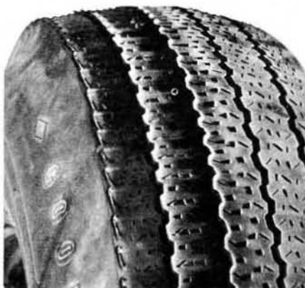
FEATHERING DUE TO MISALIGNMENT OR SEVERE CORNERING
