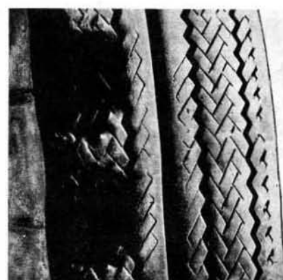
CUPPING—UNDERINFLATION AND/OR MECHANICAL IRREGULARITIES
